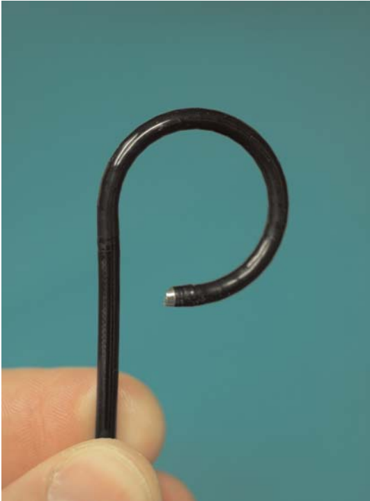
Figure 1 Flexible endoscope with a flexion of 270 degree (Richard Wolf GmbH, Knittlingen) Picture: S. Lahme
